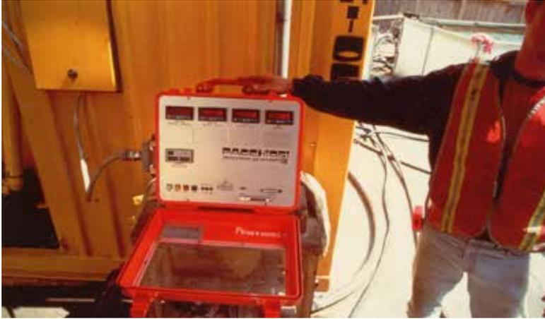
Fig. 8. PRS3 data acquisition system.
